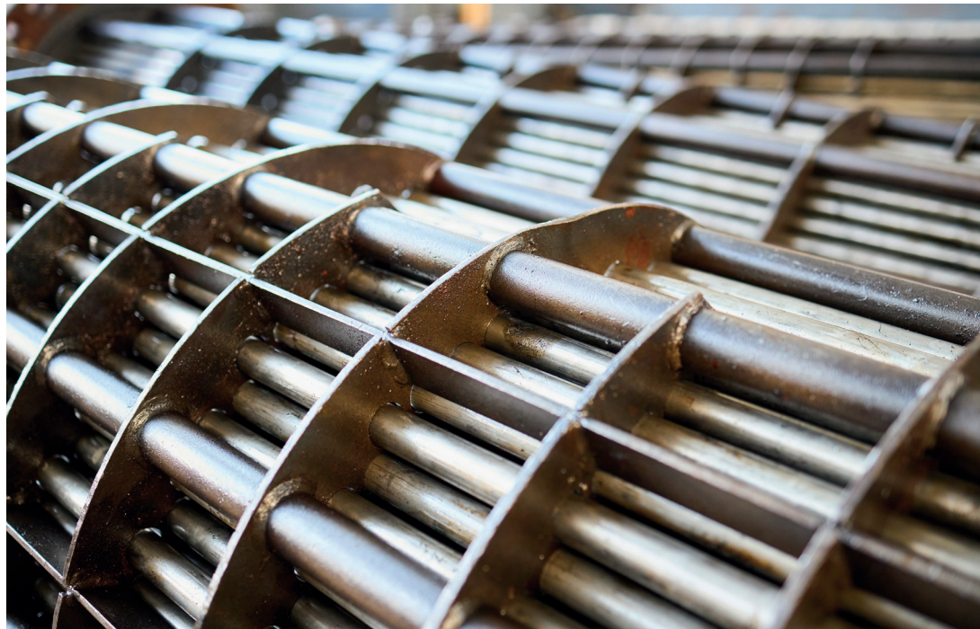
▲ Inside view of the carbon steel tube bundle within a heat exchanger.
