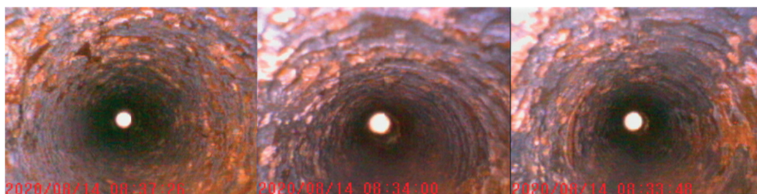
Figure 4. Erosion/corrosion problems in Cu-Ni tubes. Presence of dispersed sand in cooling water.
