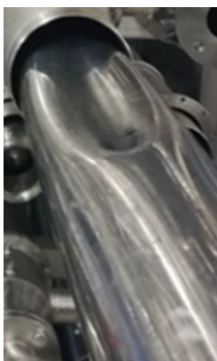
Figure 14. Collapse of a pipe due to freezing of retained water.
