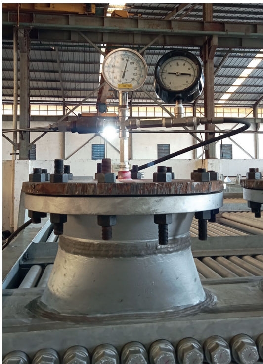
➤ Closeup of pressure gauges for hydrotesting of heat exchangers. Image courtesy of Tiga Ombak, Cortec® Case History 852.
