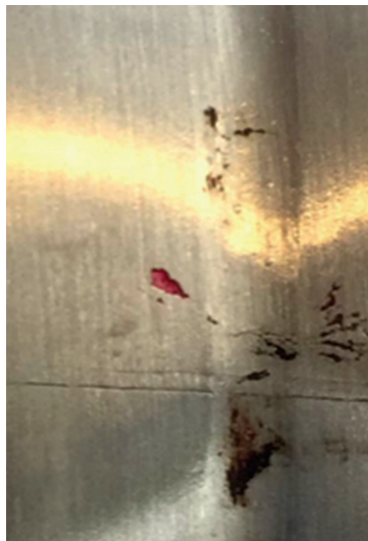
Figure 12. Beginning of corrosion attack.
