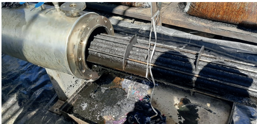
Figure 11. Example of fouling in shell side.
