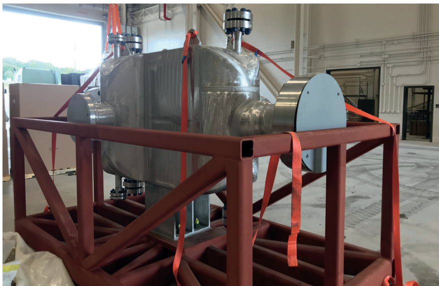
▲ The Heatric "Main Cooler" PCHE after on-site delivery to the 10 MWe STEP Demo project in San Antonio, Texas.
