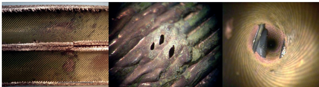
Figure 2. Overvelocity damage in copper tubes of a chiller condenser. Note how the presence of the fragment of plastic material (coming from an evaporative tower) stuck in the spiral of the pipe was the cause of the problem.
